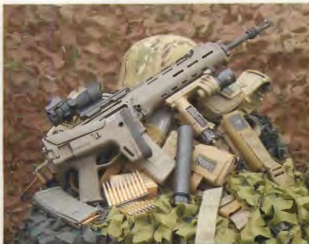
Here the Masada is seen with its stock folded. The stock is also adjustable for length of pull and height. The suppressor is by Advanced Armament.
